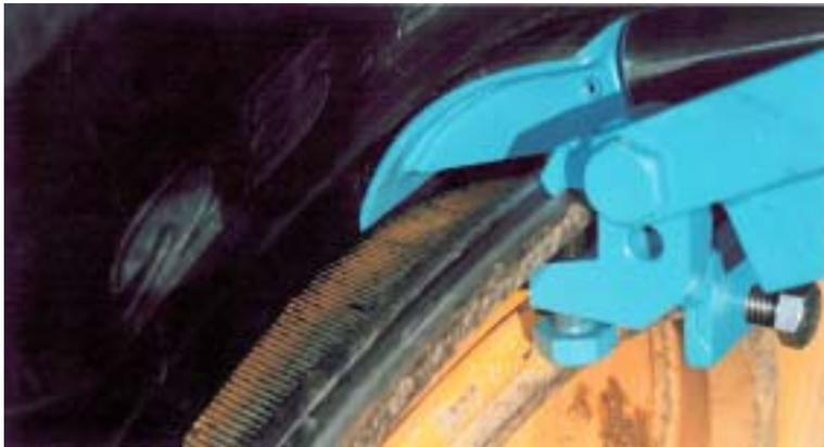
**7/** Verify that the spatula go down right up to against the rim. Proceed by little successive strokes of pump. If the spatula begins to push away the heel of the tyre, before it arrives at the stop against the wheel, release a little the hydraulic pressure, tip up the jack to the top and put the pressure again. This is necessary to oblige the spatula to go down against the wheel before it begins to push away the heel.
